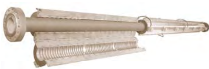
Caloritech™ Clamp-On Heater System • 58 kW, 250°F / 3500 psig, 15 W/in 2
